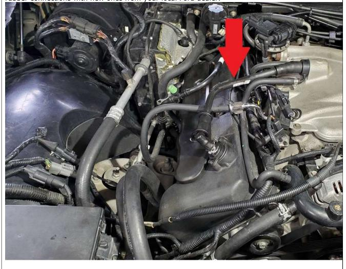
Mount J&L Bracket with supplied bolt to existing hole on front timing cover. Page 1 of 3
