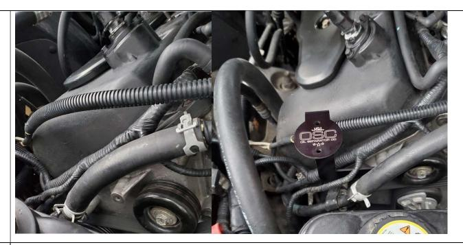
Mount J&L Oil Separator to the bracket with the supplied screws. Rotate PCV connection on valve cover to face oil separator. Lubricate connections with grease or light oil, this will help them slide fully into place. Hoses on the oil separator can twist on their respective fittings to change the angle of the hose for better layout.
